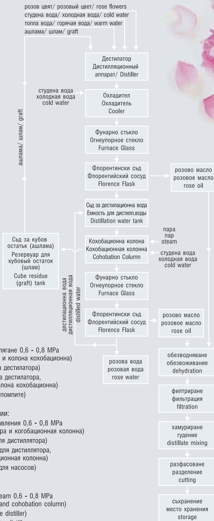
Схема на технологичния процес за производство на розово масло Schema technological process of rose oil production Diagram of the technological process for rose oil production
